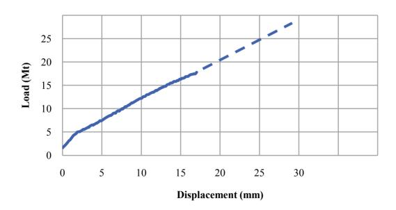
Laboratory test with a 2' (610mm) cable anchored in an dia. 2-1/4" (Ø57mm) steel tube
