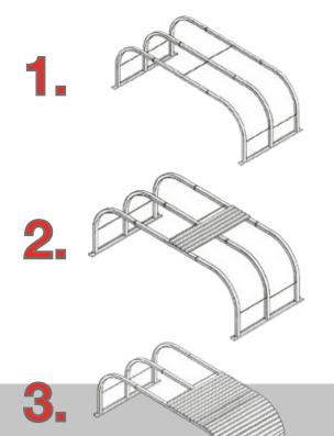
The DSI EZ Overcast provides a time tested, versatile, ventilation component for integration into any of your mining ventilation appliance needs. These overcast deck and wall structures are constructed of rolled wide flange beams in combinations of both width and height dimensions that will suit nearly any mining condition.
