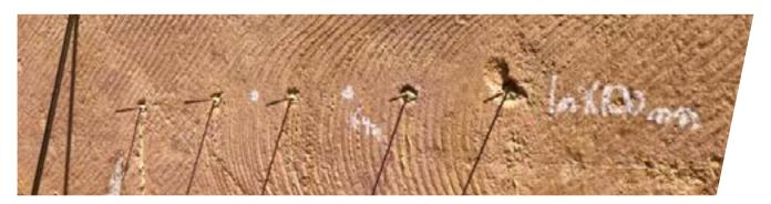
Resin Injection type bolting is an excellent new technology that can significantly increase safety and speed up development. In many instances, it can greatly improve rock support in in all sorts of ground conditions. The most interesting such system is DSI's silicate resin that we call "Mineral Bolt" resin.
